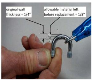
Note: For clarity the seat ubolt is shown without the seat. Also, although just one end of the chain is shown above, both ends would have to inspected.
