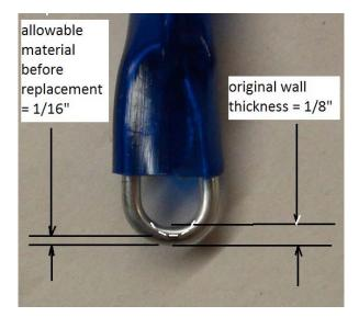
Wear in these areas are normally very light, but still should be checked. The following images show where to look for the wear and how to gauge the need for replacement. If any are found to have worn half way through the wall thickness, they need to be replaced. Remember, the simple rule to go by is "THE TIME FOR IT
